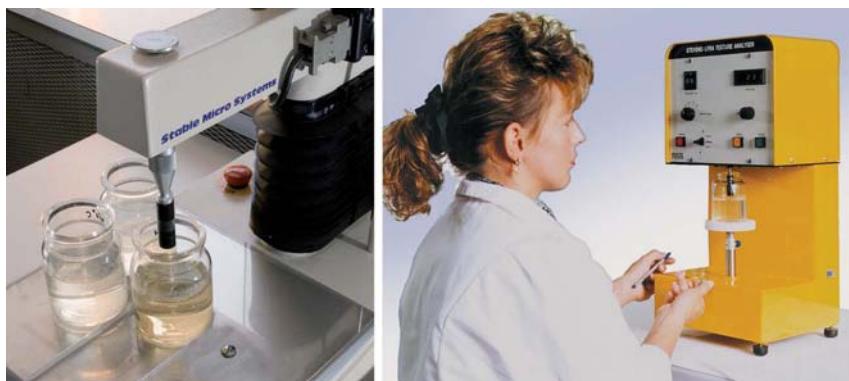
Fig. 2.53 Two different modern testing instruments for Bloom measurement.
