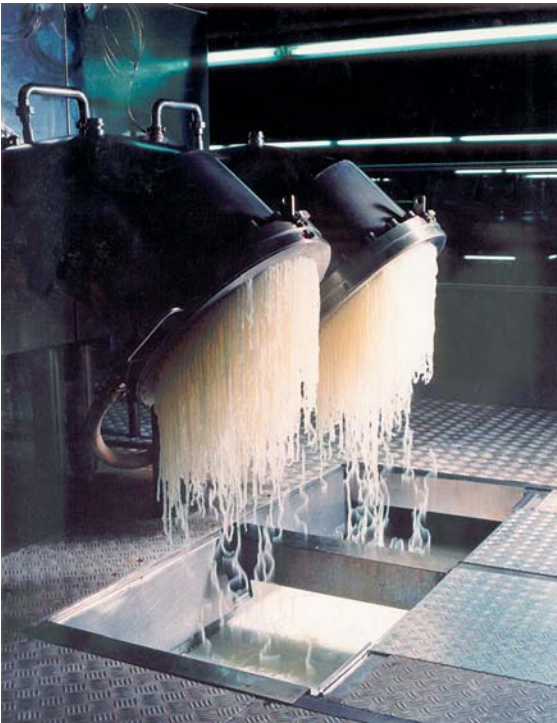
Fig. 2.37 After chilling the highly concentrated solution, the gelatine is extruded from the heat exchanger in the shape of “noodles”, which are then fed onto the conveyor belt of the drier.
