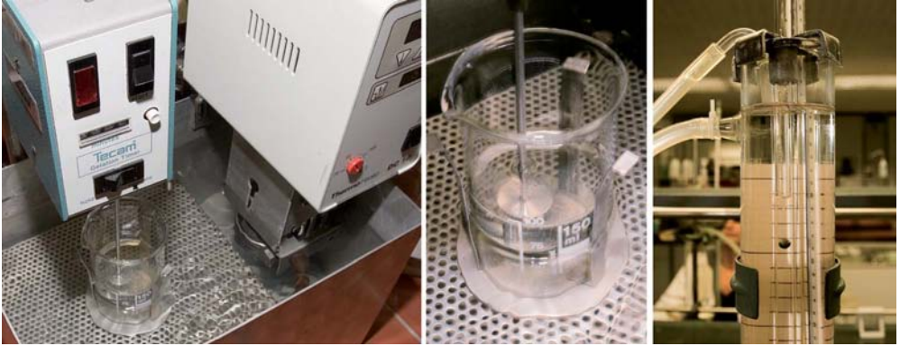
Fig. 2.59 Tecam Gelation Timer (left and center) and the glass tube method (right) for the measurement of setting time.
