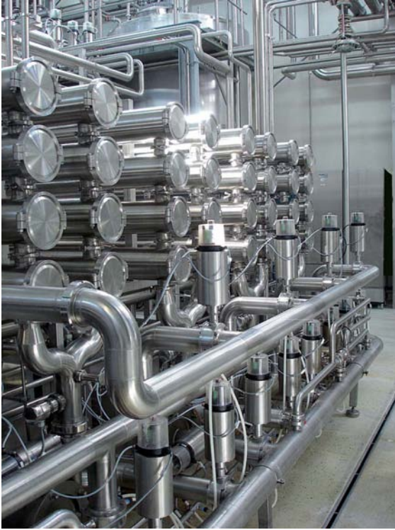
Fig. 2.33 Membrane microfiltration plant for the filtration of low molecular weight gelatine.
