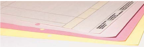
Fig. 1.10 Carbonless paper forms are covered on the back with gelatine microcapsules filled with ink. The capsules collapse and release the incorporated dye as a result of the pressure of the pen when writing.
