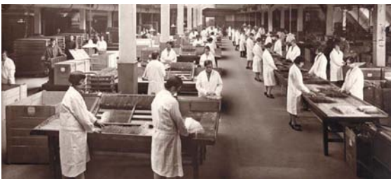
Fig. 1.3 Manufacture of gelatine was extremely work-intensive until the middle of the 20th century. Here, packing of the dried gelatine sheets.
