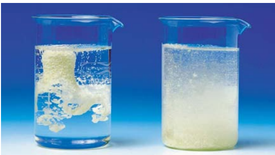
Fig. 3.34 Agglomerated gelatine hydrolysates (right) tend to clump less. They can therefore be dissolved more easily than standard types.
