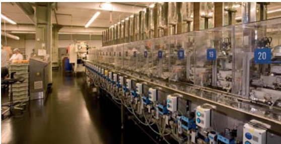
Fig. 2.41 Automatic counting and packaging line for leaf gelatine.
