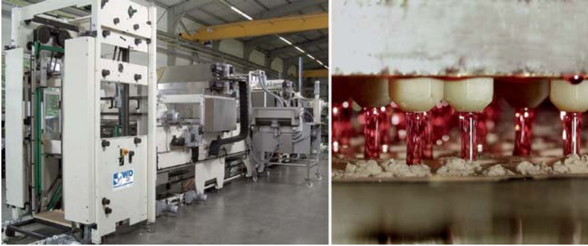
Fig. 3.38 The slurry is molded into forms (right) using a Mogul machine (left).
