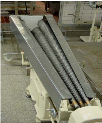
Fig. 3.39 Cone roller for the forming of fruit chews.
