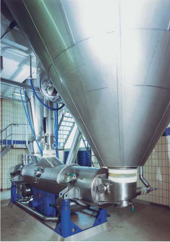
Fig. 2.48 Spray-drier with added agglomeration unit for the production of gelatine hydrolysate.
