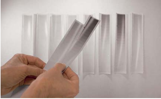
Fig. 2.63 The photographic behavior of gelatine is tested with sensitometer strips after exposure and development.
