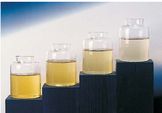
Fig. 2.28 Increasing color of the extracted gelatine, depending on the extraction step. (first extraction top right.)
