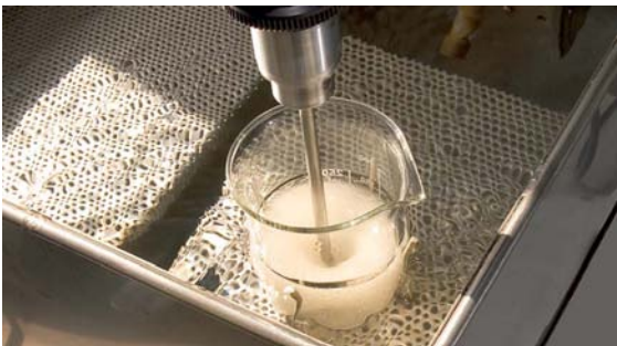
Fig. 2.64 Testing the hardening behavior of gelatine with the vortex test.
