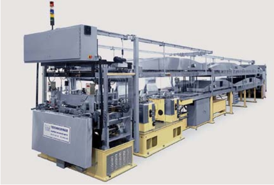
Fig. 3.72 Modern high-performance hard shell capsule machine.
