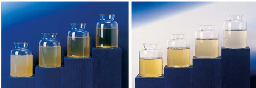
Fig. 2.56 The clarity and color of a gelatine solution are measured either visually or using appropriate equipment.
