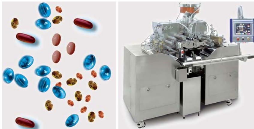
Fig. 3.77 Soft shell capsules are produced, filled and sealed in one production step. They are completely closed units in different forms and colors. On the right a modern Scherer Rotary Die machine.
