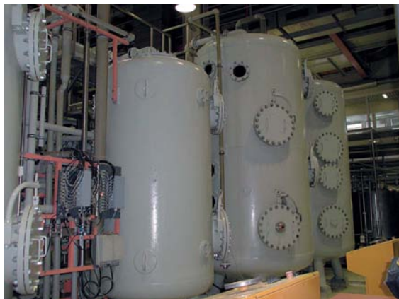
Fig. 2.34 Ion exchangers in large columns specifically remove cations or anions or deionize the gelatine solution completely.
