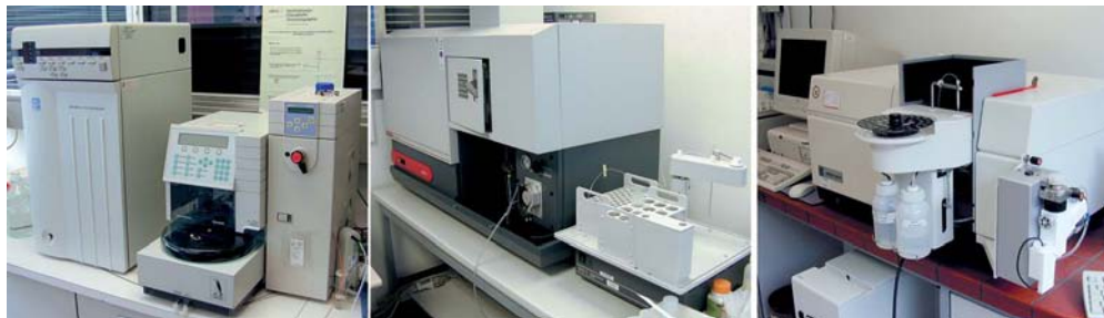
Fig. 2.57 HPLC, ICP and AAS (from the left) for the selective identification of inorganic gelatine components such as heavy metals, cations and anions.
