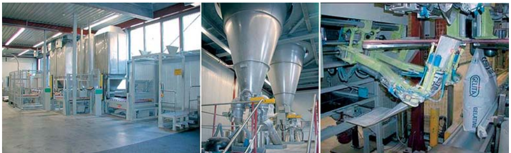
Fig. 2.39 Semi-automatic blending and packaging stations for granulated gelatine.
