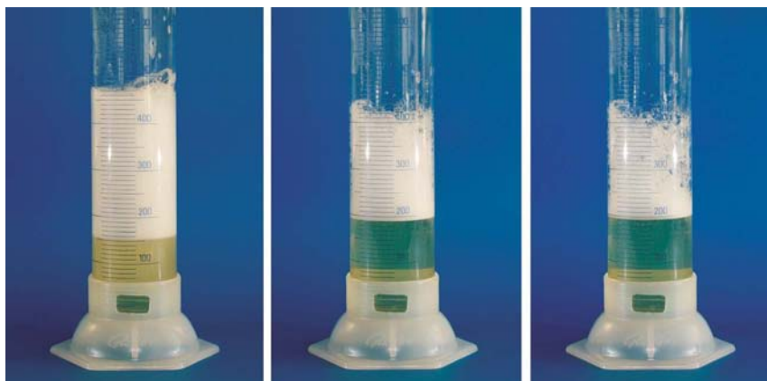
Fig. 2.61 Determination of foaming power with the perforated disk whipping method. (Left: immediately center: after 10 minutes, right: after 20 minutes.)
