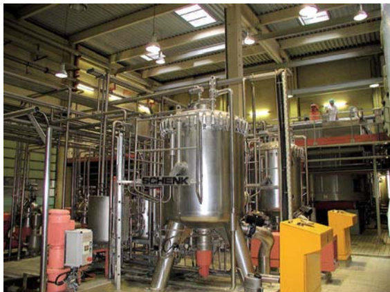
Fig. 2.32 Modern centrifugal alluvial filter equipment. Several subsequent filtration steps ensure the produced gelatine is pure.
