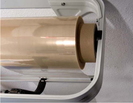
Fig. 3.111 Gelatine is a biodegradable alternative to many of today's synthetic materials. Completely biodegradable transparent films for foodstuff packaging for example have already been successfully produced.
